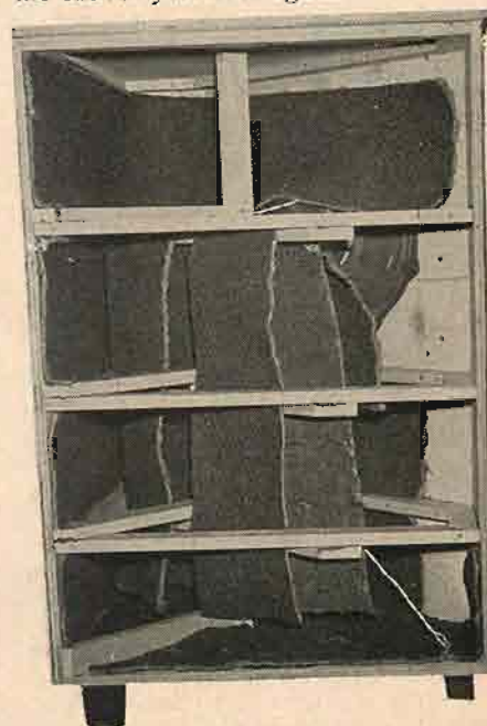
Fig. 4. Scrap strips of Ozite lining are draped over internal bracing to further dampen the cabinet.
