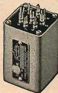
HIGH-FIDELITY INPUT TRANSFORMER, WF-20, for low impedance microphone, pickup or line to grid. Primary impedance 50, 125/150, 200, 250, 333, 500/600 ohms. Secondary impedance 50,000 ohms. Frequency response 30-20,000 cps. ± 2 db. Negligible harmonic and intermodulation distortion. Grey enamel cast case with phenolic terminal board and tapped holes for flush mounting. 2" high by 1½" square.
