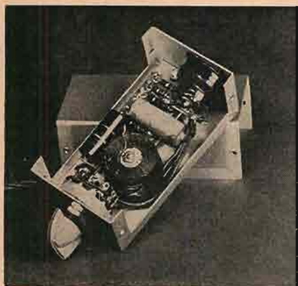
Fig. 5. Internal construction of the equalizer shown at the right in Fig. 4.
