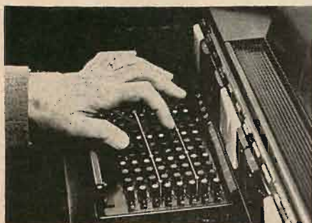
Fig. 2. The chord section is operated by 96 buttons, providing eight chords for each of the twelve keys in an octave.
