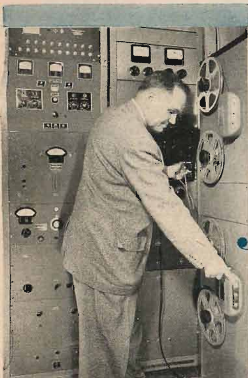
An Ampex Automatic Station now in operation at KEAR in San Mateo, California. It sustains the evening programs on tapes prepared by the daytime staff.
