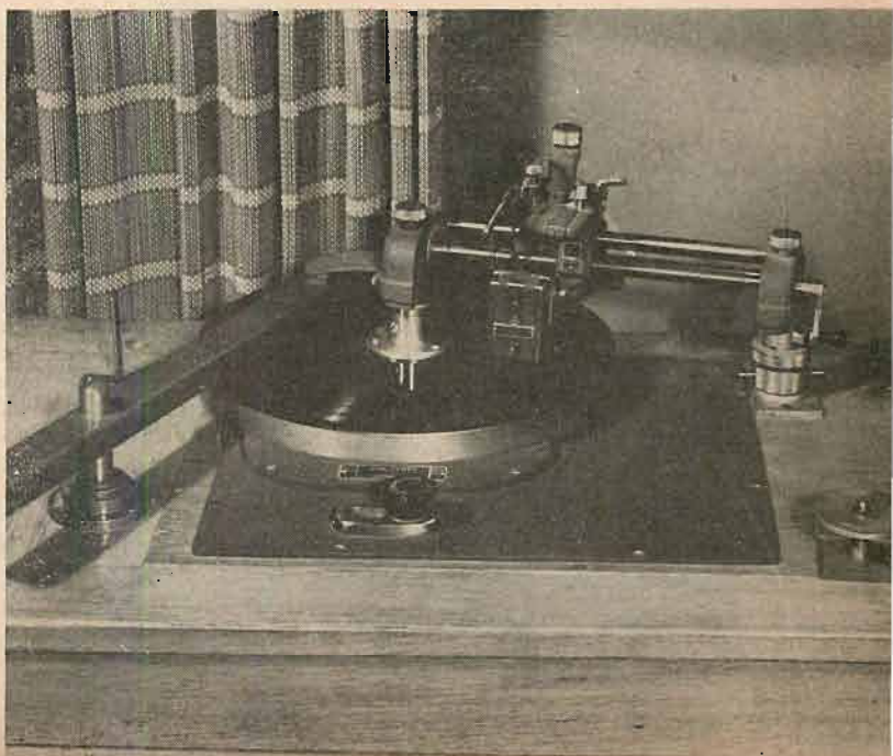
Fig. 5 (left). Shows cordsets used in hook up of output of tape recorder to input of recording amplifier, with Permoflux headphones positioned for cuing through monitor jack of tape recorder. Fig. 6 (right). Close up of Rek-O-Kut cutting lathe mounted with Presto recording head. Discs are micro-made, in addition to usual playback of complete records.
